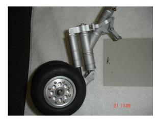
11. Right main gear pivot mechanism.
