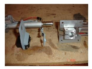
19. Bracket for direct nose wheel steering servo.
