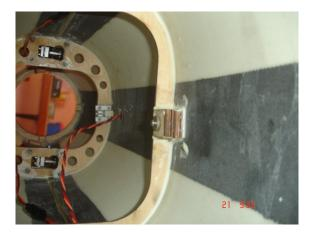
40. Fin installation bolt and fitting.
