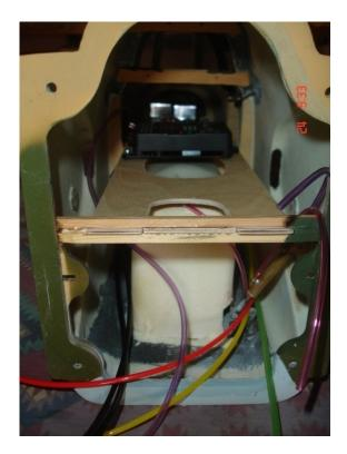
26. View into nose section from the rear showing the shelf where the Power Box (towards front) and the Turbine ECU (towards the rear) will be installed. Optional positions are above the landing gear bearer or the space behind the engine intake ducts.
