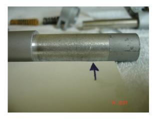
4. Point for another flat spot at the scissor link at bottom of nose gear.
