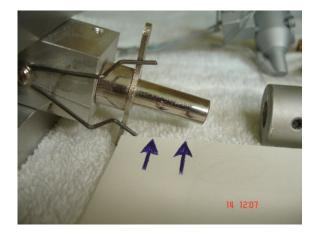
3. Nosewheel steering arm where I filed flat spots.
