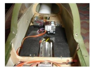
25. View into nose section showing brake air bottle for brakes and Jet Tronic valves.
