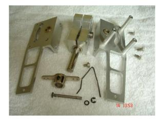
6. Nosewheel retract disassembled.
