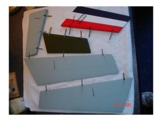
15. Hinges installed on control surfaces.
