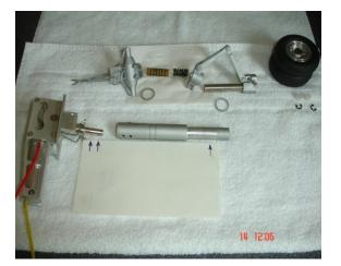
2. Nosewheel disassembled.
