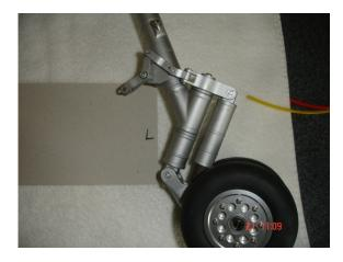
10. Left main gear pivot mechanism.
