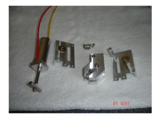
12. Main gear retract unit disassembled.
